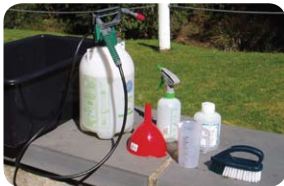
Field washdown equipment for simple field activities – spray bottles, footbaths, gloves, brush, disinfectant, measuring device. Photos courtesy of DPIPW Water Assessment and Hydro Tasmania.
