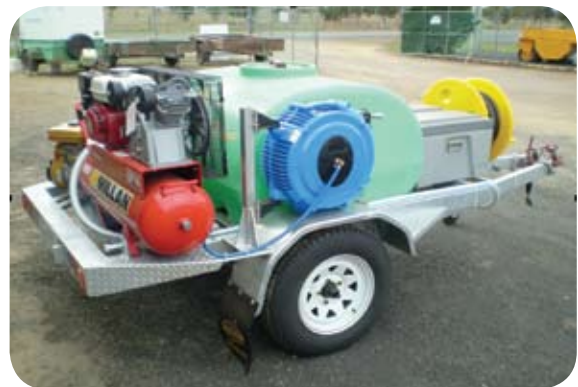
Mobile washdown unit with high pressure pump, hose and compressed air unit. Photo courtesy of NRM South/Southern Tasmanian Councils Authority.
