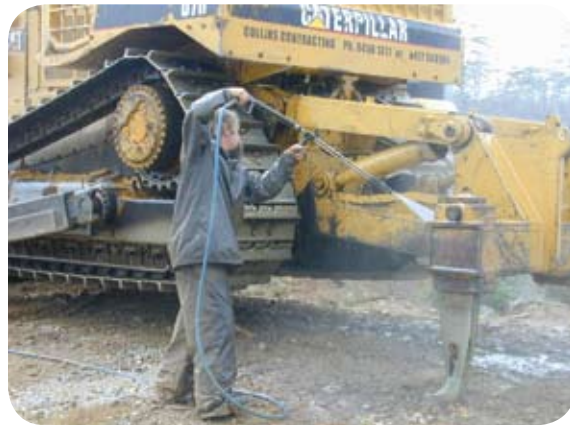
After physical removal of soil and dirt a high pressure hose is used to further remove clods. Machinery has been elevated with boom arm to enable cleaning underside. Photo courtesy of Forestry Tasmania.
