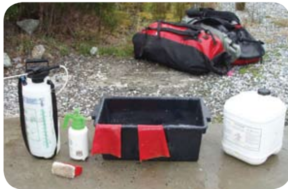
Field washdown equipment for simple field activities – spray bottles, footbaths, gloves, brush, disinfectant, measuring device. Photos courtesy of DPIPW Water Assessment and Hydro Tasmania.
