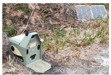
The Felixer cat grooming trap is a new and innovative method for controlling feral cat populations. The device contains a camera, data processing unit and cartridges of 1080 poison.
