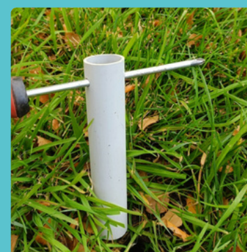
Removing PVC pipe using screwdriver
