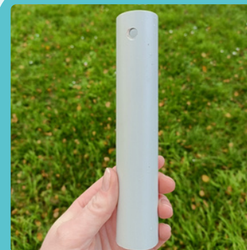
15cm PVC pipe, with 2 small holes
